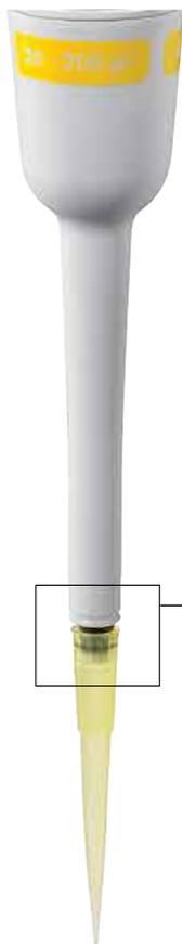
Two optional accessories are available for the single-channel Transferpette® models with volume ranges of 20-200 µl and 100-1000 µl. One is a patented shaft tip that is co-molded of hard and resilient components. Also available are three ejector clips. These ensure that tips are not mounted with more force than needed to seal, so that tip ejection will take only a light touch.
